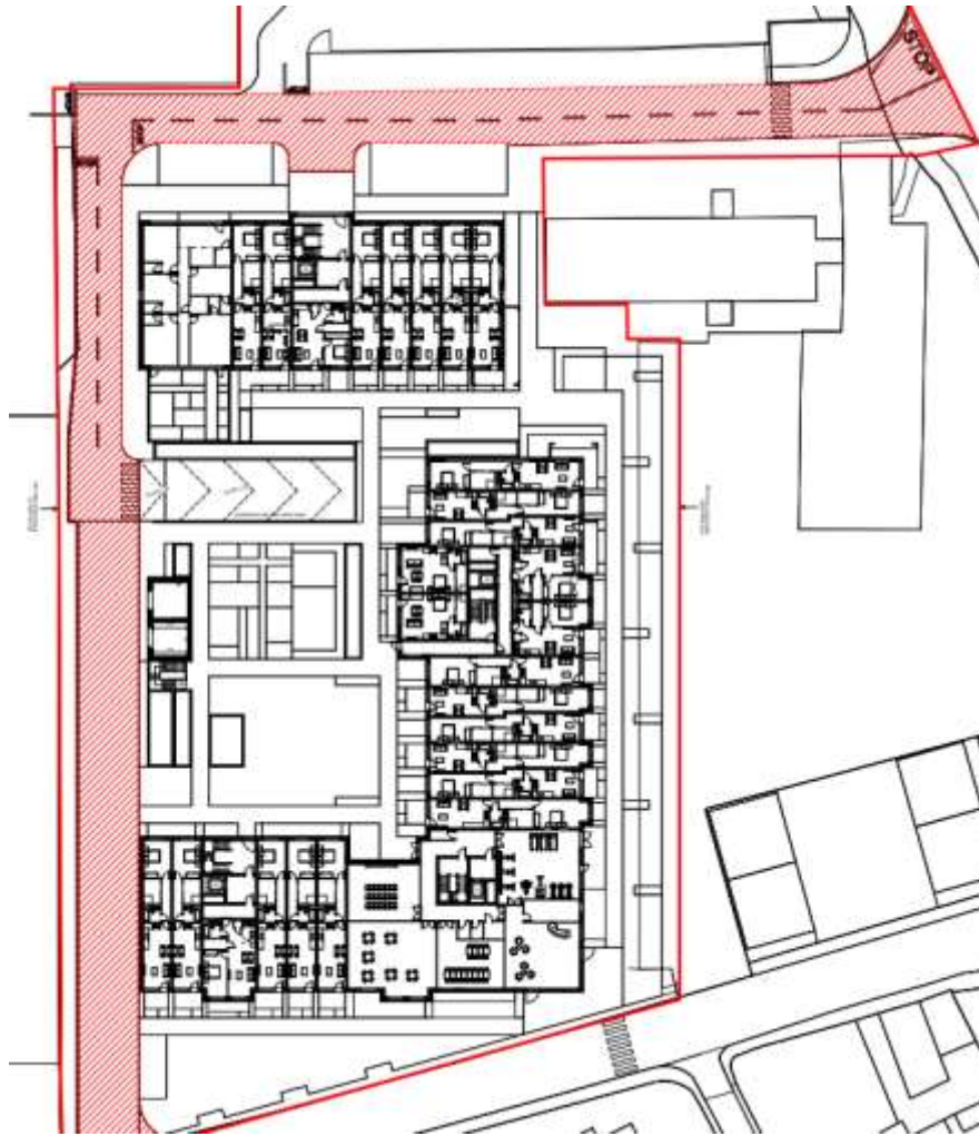
Fig. 3 Taking In Charge plan (red hatch areas to be taken in charge)
