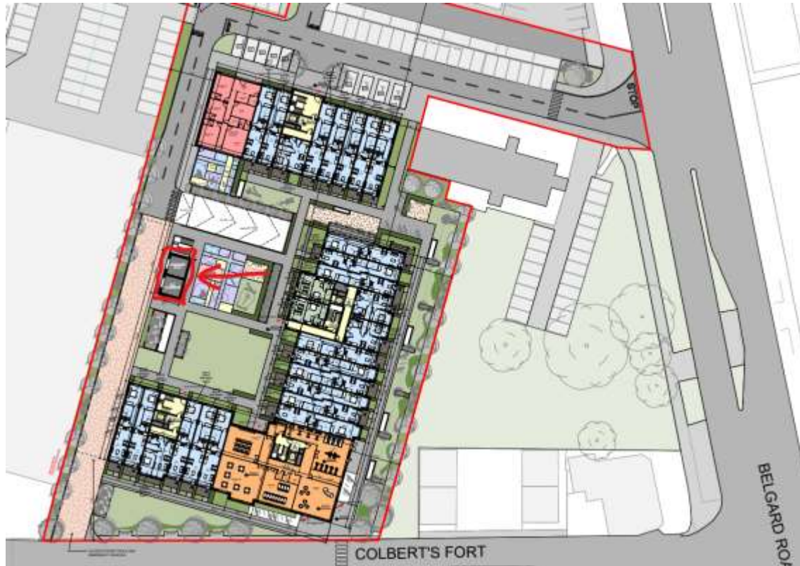
Ground floor plan indicating ESB Substation location
